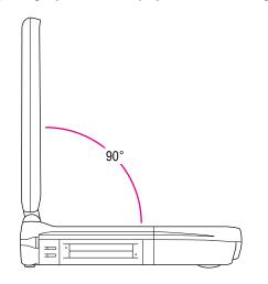
6 While holding the keyboard in place, rotate the PowerBook so the that underside faces up, with the display flat against the table surface.
